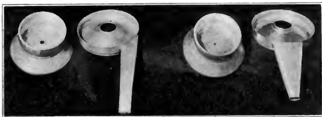
FIG. 3.—LEFT, BOWL PARTS USED IN SEPARATING NORMAL CREAMS; RIGHT, THOSE FOR SEPARATING HIGH-TESTING CREAMS, FARM-SIZE SEPARATOR
